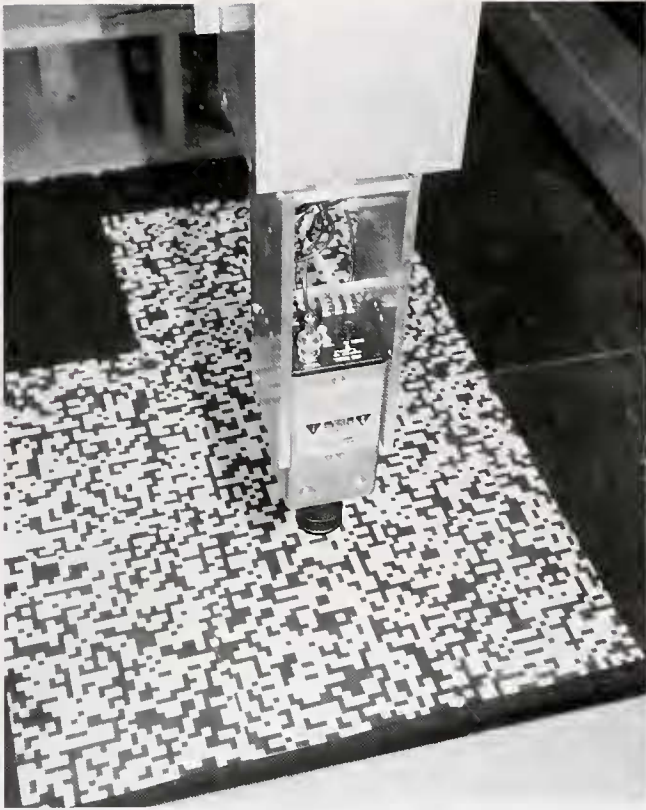
Figure 3. View of robotic gantry, showing camera head and visual texture on the floor. Adapted from Srinivasan et al. (2000).
